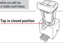
Remove the Inlet Cap and fill the Ice Canister halfway with ice through the Ice/Salt Inlet. This is indicated by the ICE and SALT marker on the Canister
